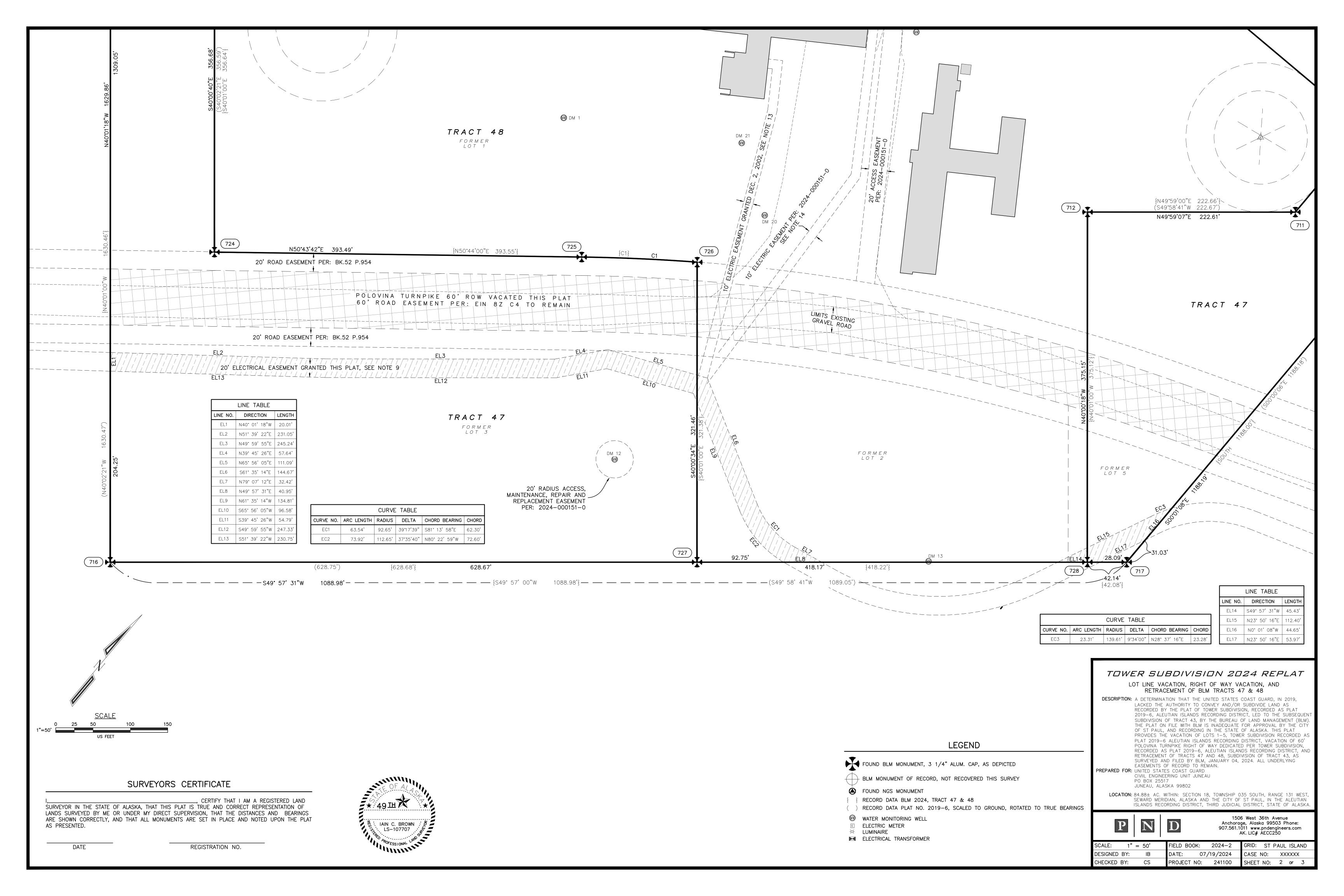
THE VERTICAL DATUM FOR THIS SURVEY IS NORTH AMERICAN VERTICAL DATUM OF 1988 (NAVD88), BASIS OF ELEVATION IS N.G.S. STATION "SOUTHWEST BASE", POINT NO. 204 THIS SURVEY. ORTHOMETRIC HEIGHT FOR 204 WAS DETERMINED VIA STATIC GNSS OBSERVATION, POST PROCESSED UTILIZING NATIONAL GEODETIC SURVEY (NGS) ONLINE USER POSITIONING SERVICE (OPUS). POINT NO. 204 WAS DETERMINED TO HAVE THE FOLLOWING ELEVATION:
